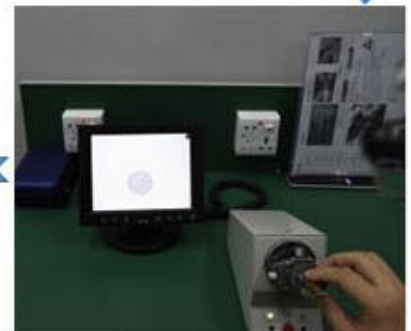
Cleaning end face
